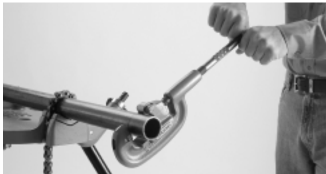
Figure 1 – Cutting End of Pipe
